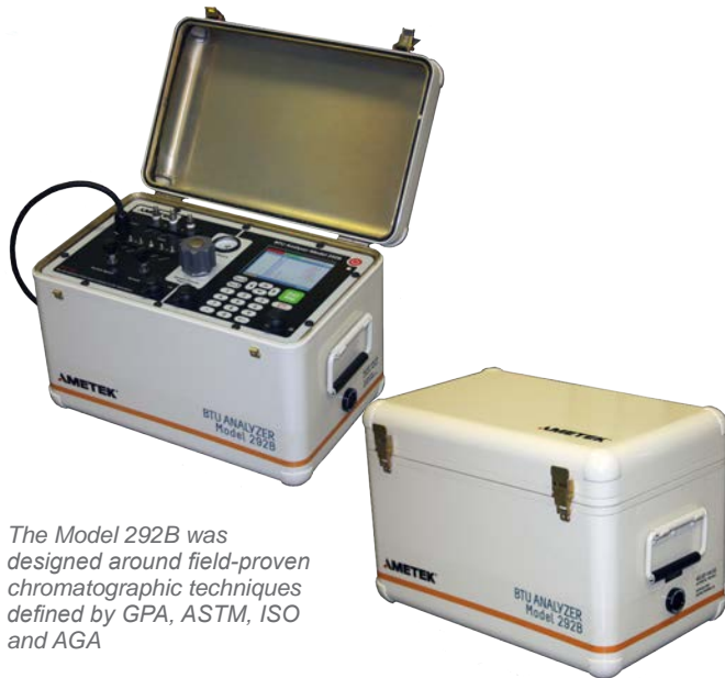
Figure 1: The AMETEK 292B Portable BTU Analyzer
