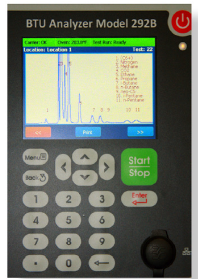
Figure 2. A Typical Natural Gas Chromatogram
