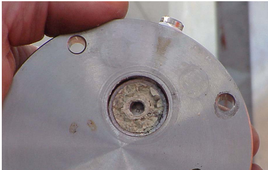
Figure 7 – Sulfur on Particulate Filter After Process Upset
