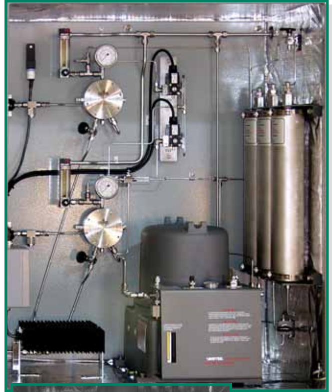
2-pt. Zone 1 Sample System (above); 4-pt. Gas Sample System (inset)
