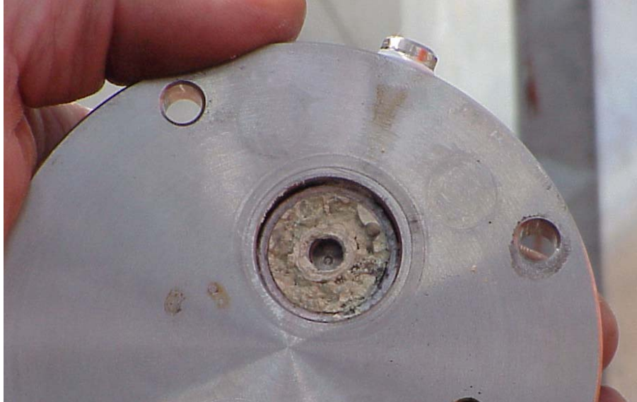
FIGURE 7 – SULFUR ON PARTICULATE FILTER AFTER PROCESS UPSET
