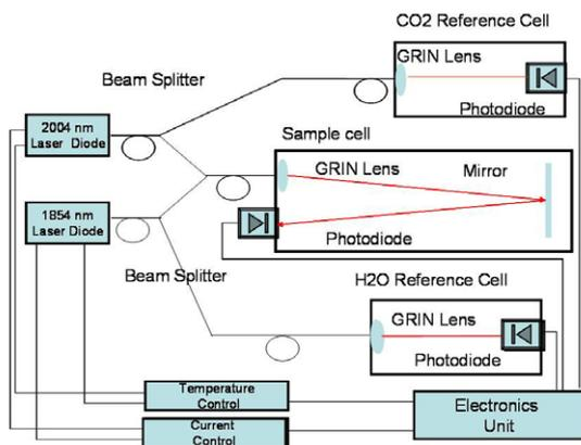
Figure 7. Multi-component AMETEK TDLAS system including built-in reference cell for system verification and line-lock capability.
