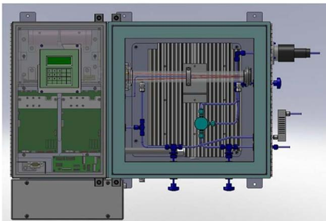
Figure 8. AMETEK Model 5100 HD analyser with sealed reference cell and built-in sample system.
