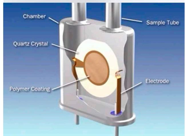
Figures 4 and 5. QCM analyser and analyser cell.
