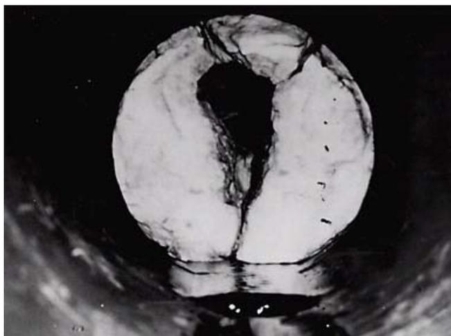
Figure 1. Natural gas hydrate, partial pipeline blockage.
