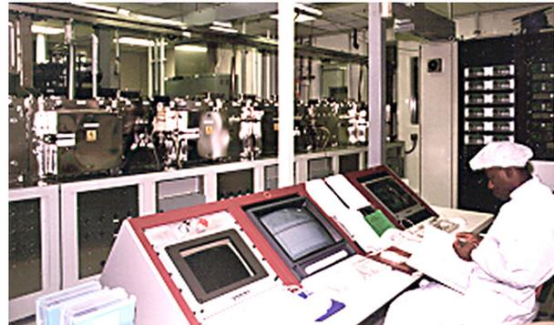
Figure 2. Dycor RGA on each chamber of the deposition system
