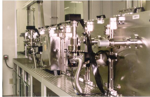
Figure 1. Seagate horizontal deposition system
