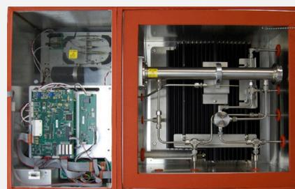
Figure 1. The AMETEK 5100HD TDLAS for water vapor in CO<sub>2</sub>
