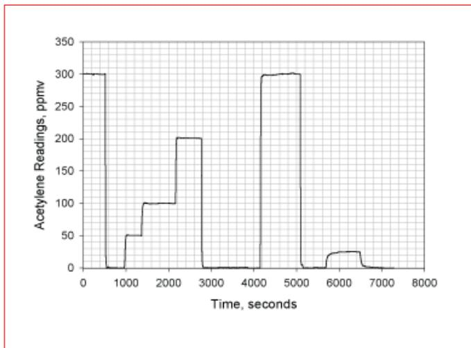
Figure 5. Typical performance in the C<sub>2</sub>H<sub>2</sub> medium concentration range
