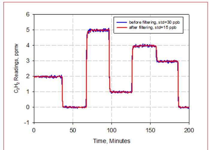
Figure 6. Low ppmv C<sub>2</sub>H<sub>2</sub> measurements in a multi-pass gas cell integrated analyzer
