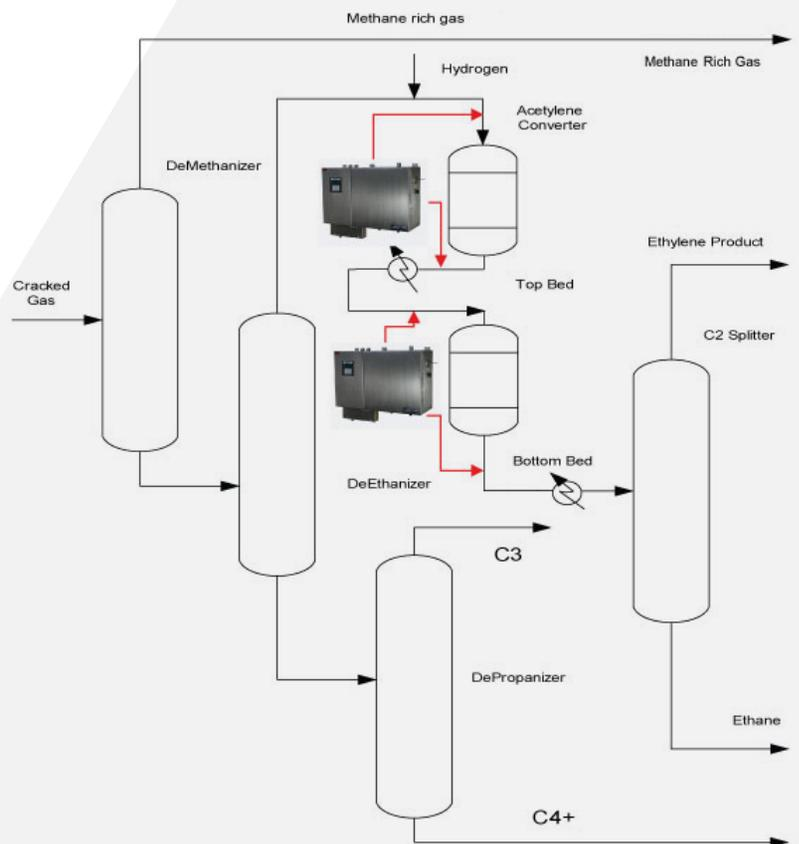
Figure 1. A diagram of a typical  $C_2H_4$  production plant and sampling points for a TDLAS analyzer
