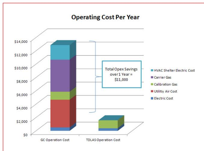
Figure 4. Operating cost of a TDLAS versus a process GC
