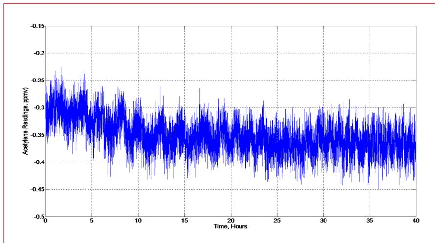
Figure 7. Instrumental drift of the analyzer over 40 hours
