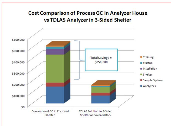
Figure 3. Capital cost of a TDLAS versus a process GC
