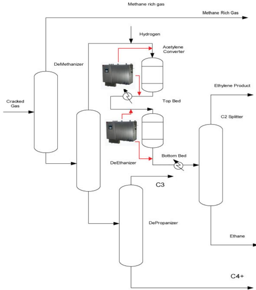
Figure 1. A diagram of a typical ethylene production plant and sampling points for a TDLAS analyzer.
