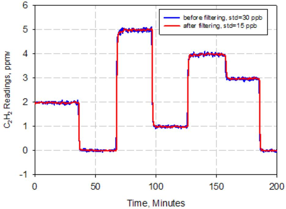
Figure 6. Typical Performance in the Acetylene Low Concentration Range
