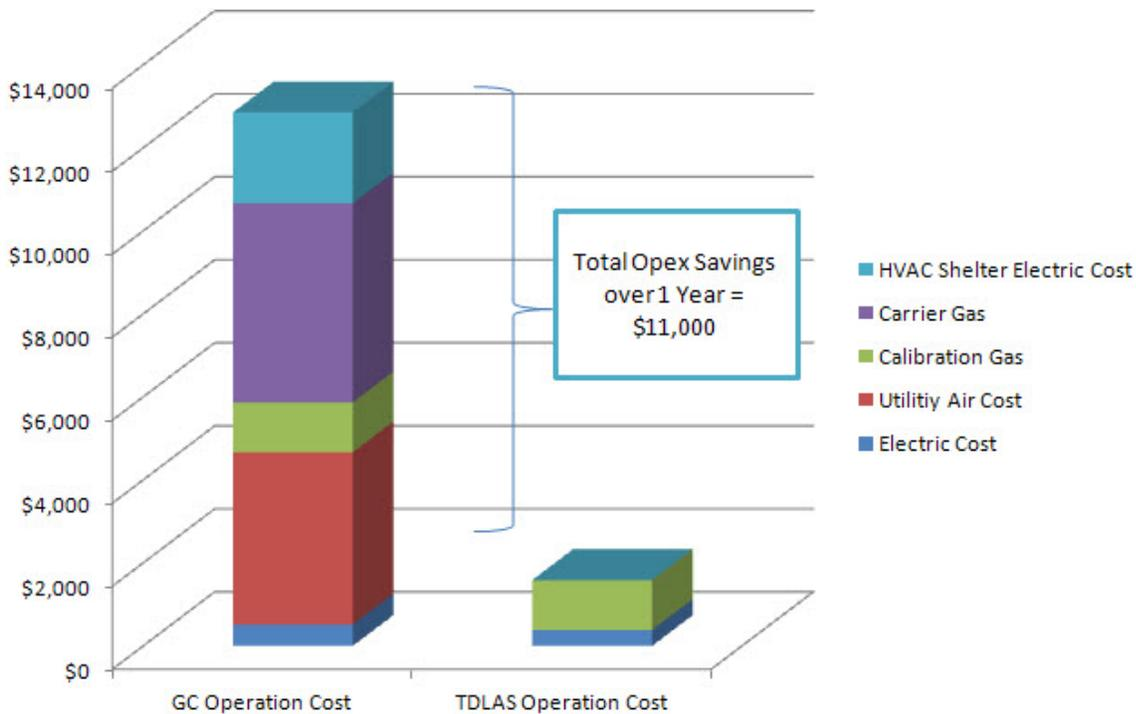
Figure 4. Operating cost of a TDLAS versus a process gas chromatograph
