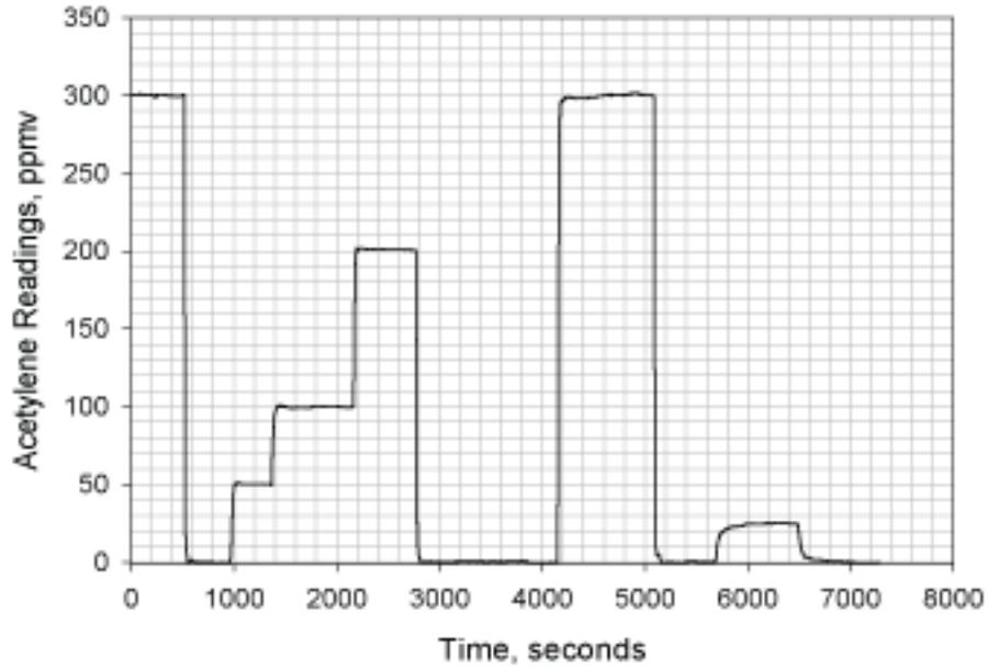
Figure 5. Typical Performance in the Acetylene Medium Concentration Range
