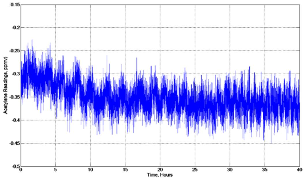
Figure 7. 40-hour Drift Measurements for Acetylene in Ethylene
