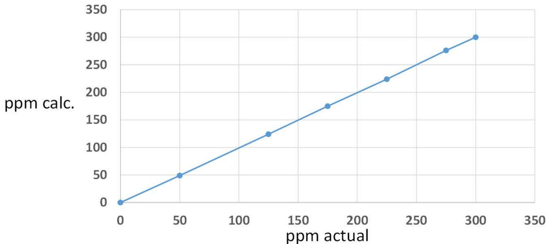
Figure 3: Validation Results for AMETEK TDLAS Measurements of Water in Hydrogen Recycle Gas
