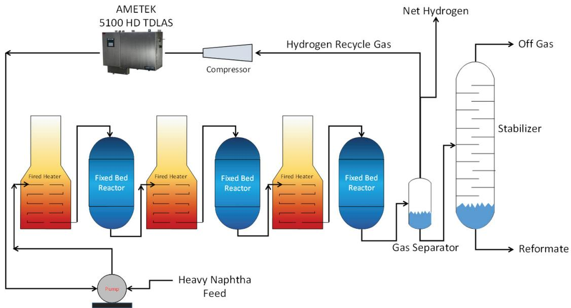
Figure 1: Diagram of a Three Bed Catalytic Reformer
