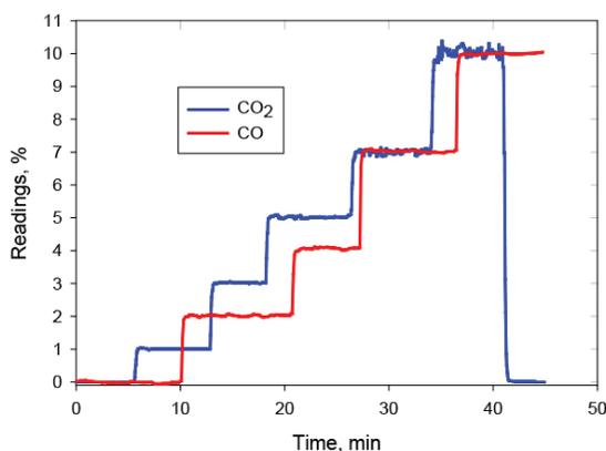
Figure 2: Response of the analyzer to a series of CO<sub>2</sub> and CO concentration challenges.
