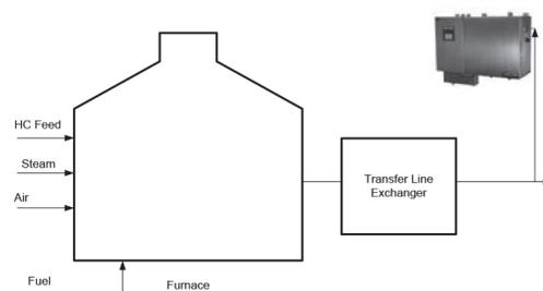
Figure 1: Monitoring of the Decoking Process in Ethylene Furnace.
