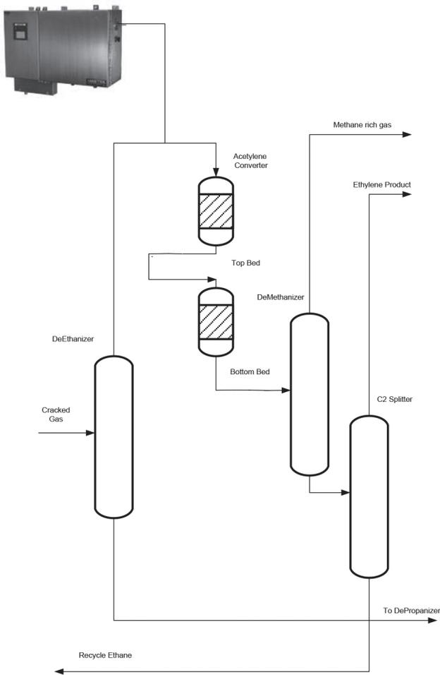
Figure 1: Front-End DeEthanizer Acetylene Hydrogenation.
