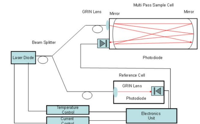
Figure 4. Diagram of a TDLAS analyzer
