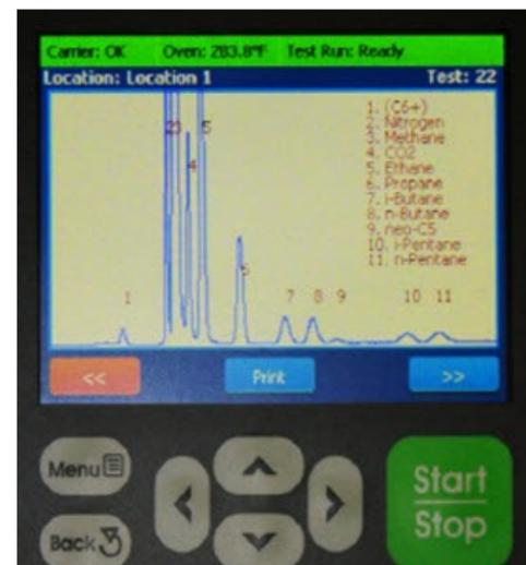
Figure 3. Control panel of a gas chromatograph
