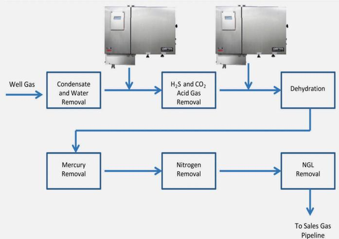
Figure 1. Diagram of a natural gas processing plant
