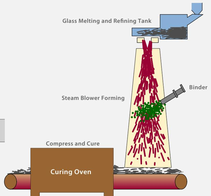
Figure 2. Glass fiber manufacture
