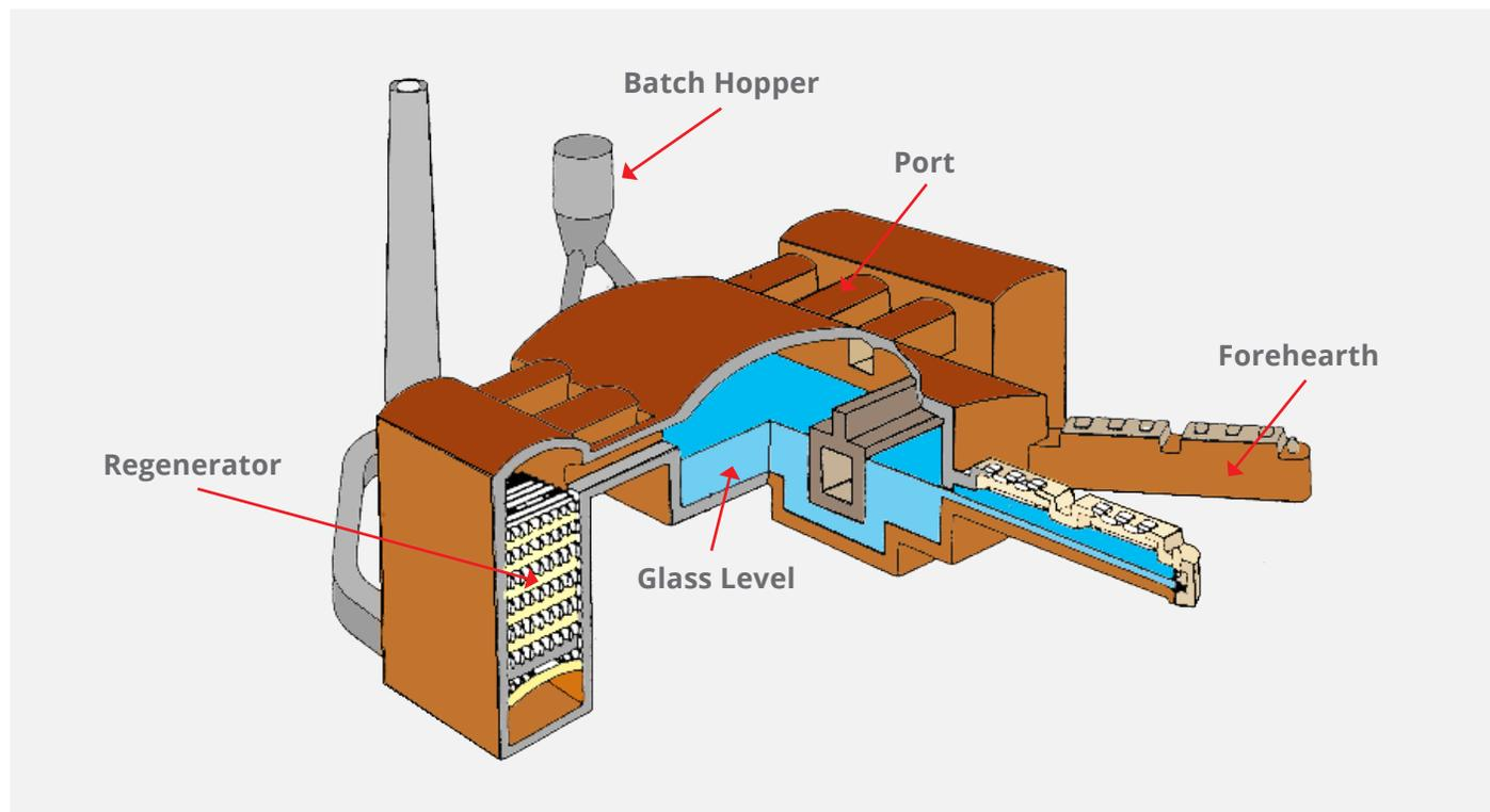
Figure 3. Glass melt tank and forehearth
