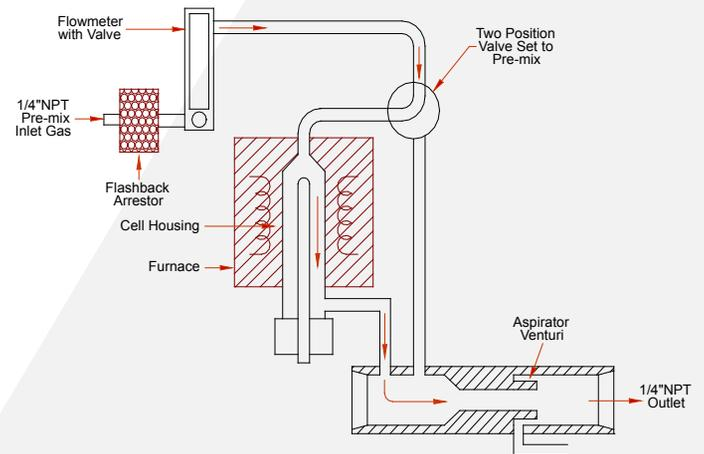
Figure 4. CMFA-P2000 flow diagram
