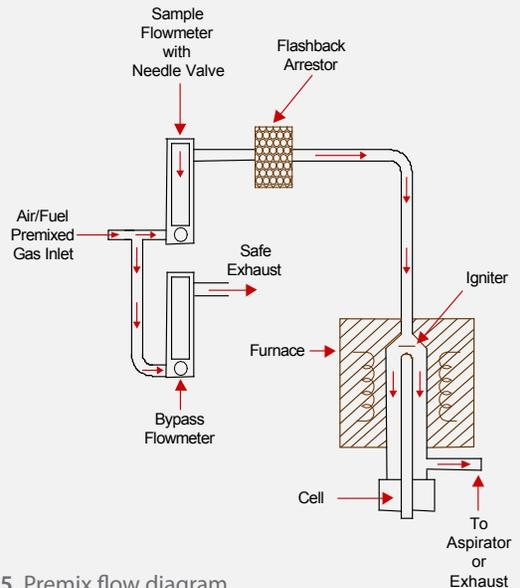
Figure 5. Premix flow diagram
