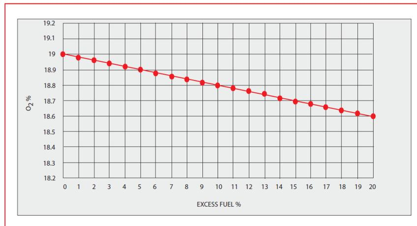
Figure 6. Oxygen in premix vs. excess fuel
