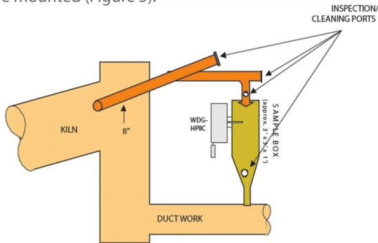
**Figure 5.** Bypass sample box
