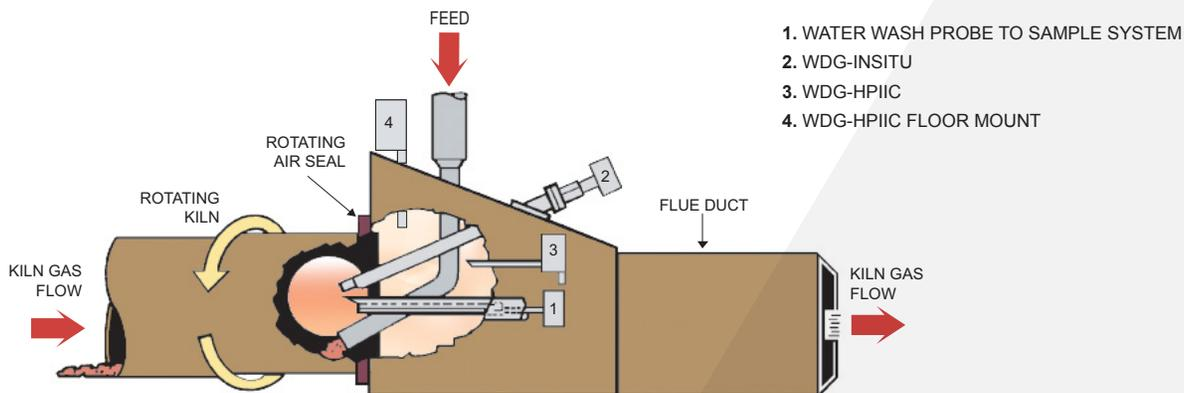
Figure 2. Various kiln measurements
