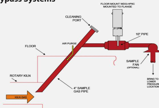
Figure 3. Bypass vertical probe
