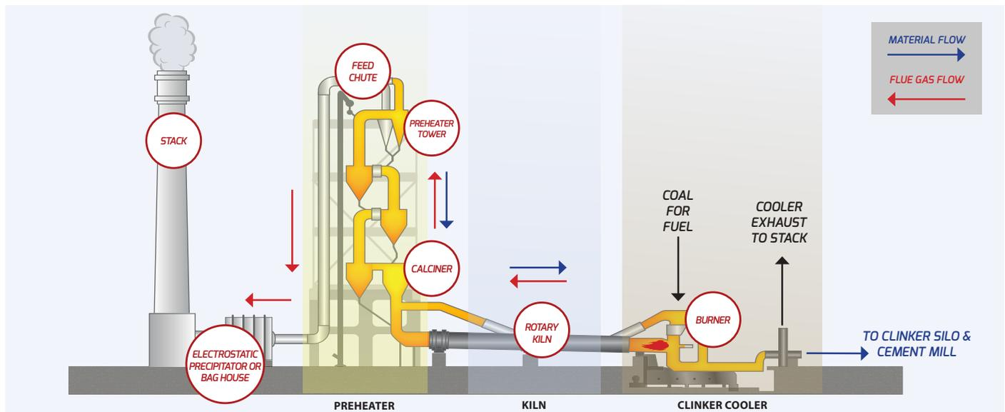
Figure 1. Cement lime process diagram
