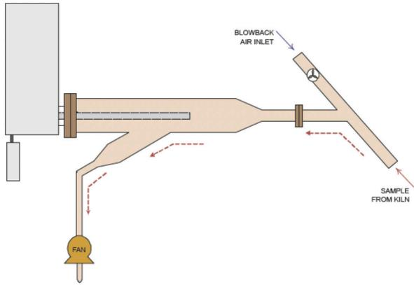
**Figure 4.** Bypass horizontal probe
