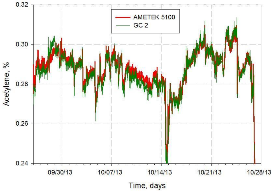
FIGURE 7. ACETYLENE MEASUREMENTS AT THE OUTLET OF THE FIRST BED OF THE CONVERTER.
